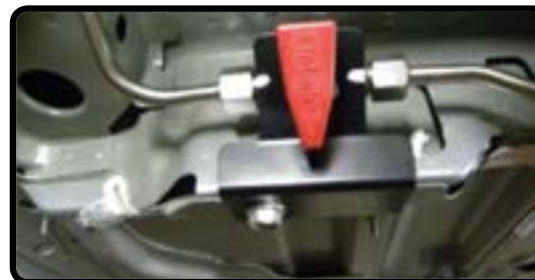
1/4 Turn Shut-Off Valve, Off Points Down
